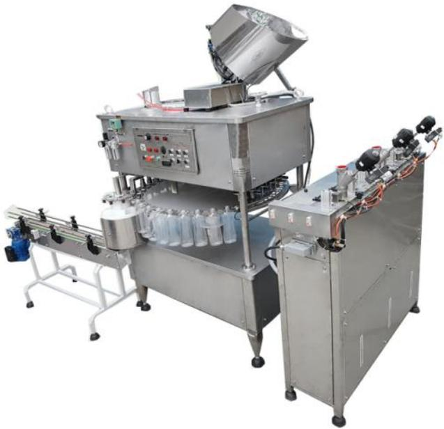
The Automatic 6-Nozzle Filling and Capping Machine with a Speed of 2000 Bottles per Hour is an industrial machine used for filling and capping various plastic, glass, metal, and other bottles. This machine uses a rotary cylinder piston mechanism to fill the desired materials into the bottles at high speed and accuracy and then seals them.
