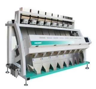
The ABT-CS8 color sorter is a grain sorting machine with a nominal inlet capacity of 9.5-12 tons per hour. It uses three-dimensional scanning technology to separate grains based on color, size, and shape. The ABT-CS8 can separate defective, damaged, moldy, and infested grains from healthy grains. This machine is used in various industries, including food, agriculture, and pharmaceuticals.
