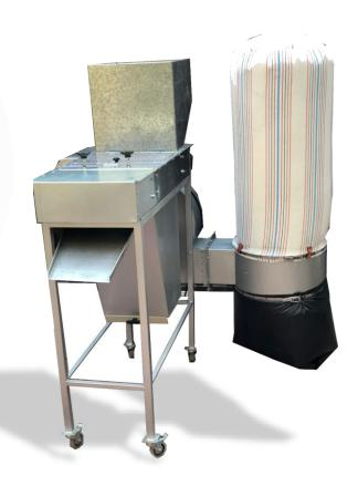
Unique features of this peanut peeling machine include a skin collection system and its guidance into the bag. With this feature, you not only provide sufficient safety for the workforce during use, but also during peeling. Also, due to the presence of this collection system, peanut and walnut peeling can be done easily and without further manipulation.
