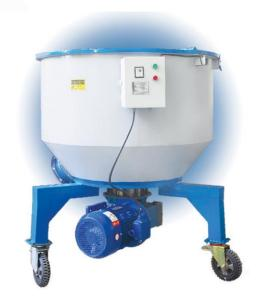
A coffee mixer is a machine used to mix coffee grounds and other powders evenly. It can be used for industrial and semi-industrial applications.
